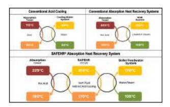
medium pressure steam. Acid at 200-225°C bottom temperatures can easily boil pressurized water at 8-10 bar or pre-heat high pressure boiler feedwater while reducing cooling water consumption and related treatment costs.
