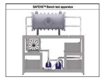
trolled by the flow of the cold fluid; the higher the flow, the more condensation and consequently the lower the internal pressure of the vessel. Safety fluid partly fills the volume of the shell, covering the hot side tubes, similar to a steam generating boiler. The top is out of contact with the liquid level and works as a condenser.
