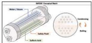
The buffer fluid selection addresses the exchanged process temperatures to give the optimal thermodynamic and chemical properties in the heat exchange working range.
